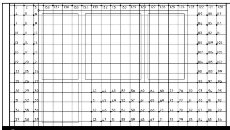
Figure 3. Mesh used to read out average temperature for small area surfaces
