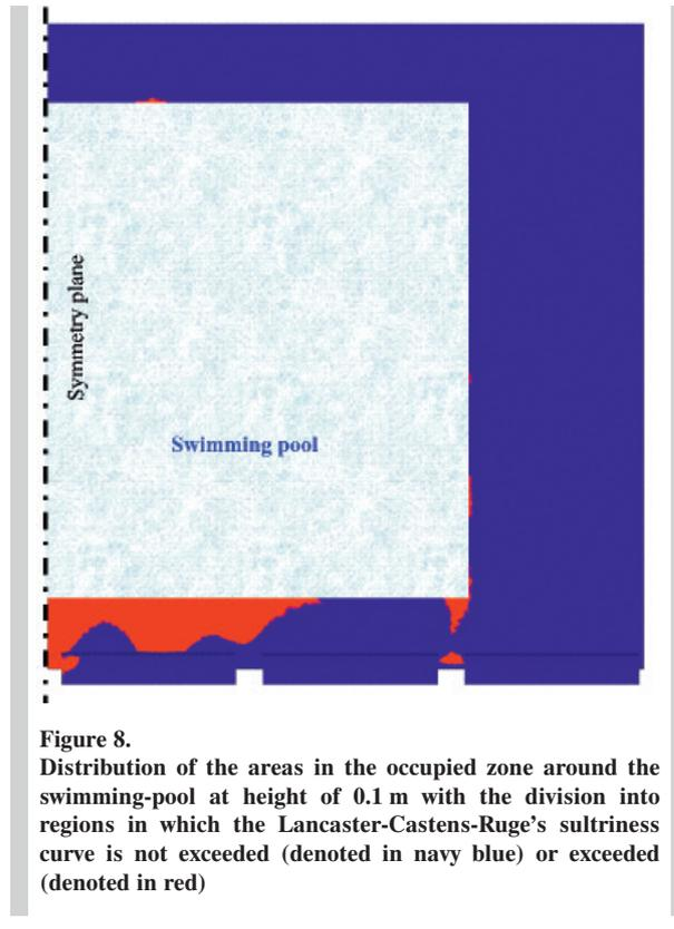
**Figure 8.** Distribution of the areas in the occupied zone around the swimming-pool at height of 0.1 m with the division into regions in which the Lancaster-Castens-Ruge's sultriness curve is not exceeded (denoted in navy blue) or exceeded (denoted in red)
