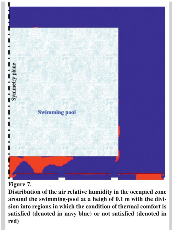
**Figure 7.** Distribution of the air relative humidity in the occupied zone around the swimming-pool at a height of 0.1 m with the division into regions in which the condition of thermal comfort is satisfied (denoted in navy blue) or not satisfied (denoted in red)
