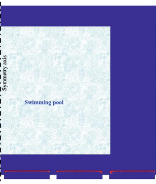
**Figure 11.** Distribution of the DR index in the occupied zone around the swimming-pool at a height of 0.1 m with the division into region in which the criterion of avoidance of local thermal discomfort is satisfied (denoted in navy blue) or not satisfied (denoted in red)
