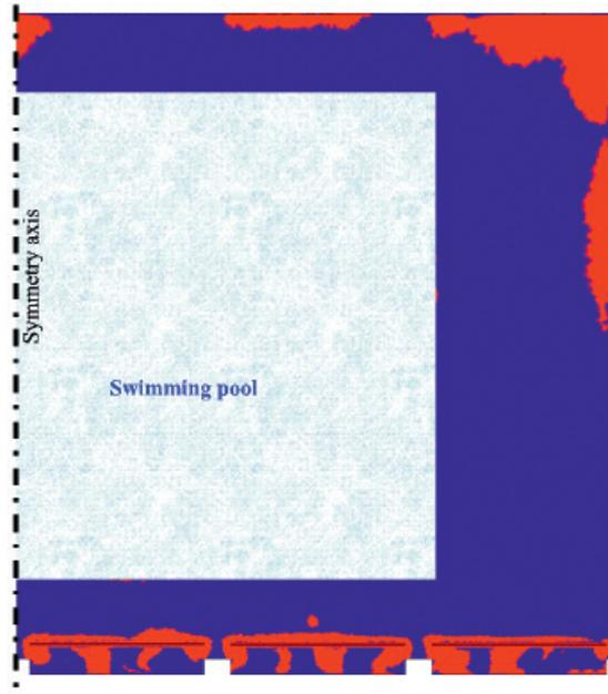
**Figure 12.** Distribution of the parameter  $\Theta$  in the occupied zone around the swimming-pool at a height of 0.1 m with the division into regions in which the conditions of the ADPI index is satisfied (denoted in navy blue) or not satisfied (denoted in red)
