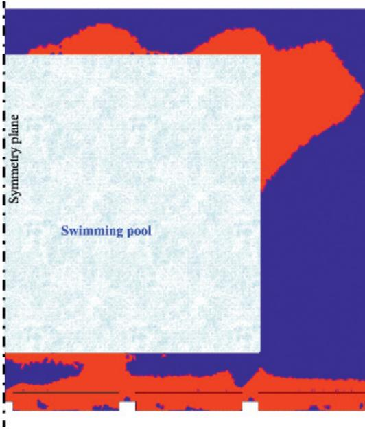
**Figure 10.** Distribution of the PMV index in the occupied zone around the swimming-pool at a height of 0.1 m with the division into regions in which the condition of thermal comfort is satisfied (denoted in navy blue) or not satisfied (denoted in red)
