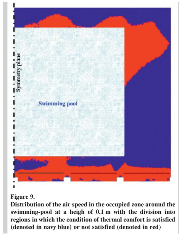
**Figure 9.** Distribution of the air speed in the occupied zone around the swimming-pool at a height of 0.1 m with the division into regions in which the condition of thermal comfort is satisfied (denoted in navy blue) or not satisfied (denoted in red)
