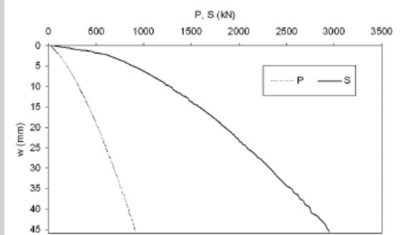
**Figure 9.** Mobilisation of loads at the base and lateral surface of jet grouting column
