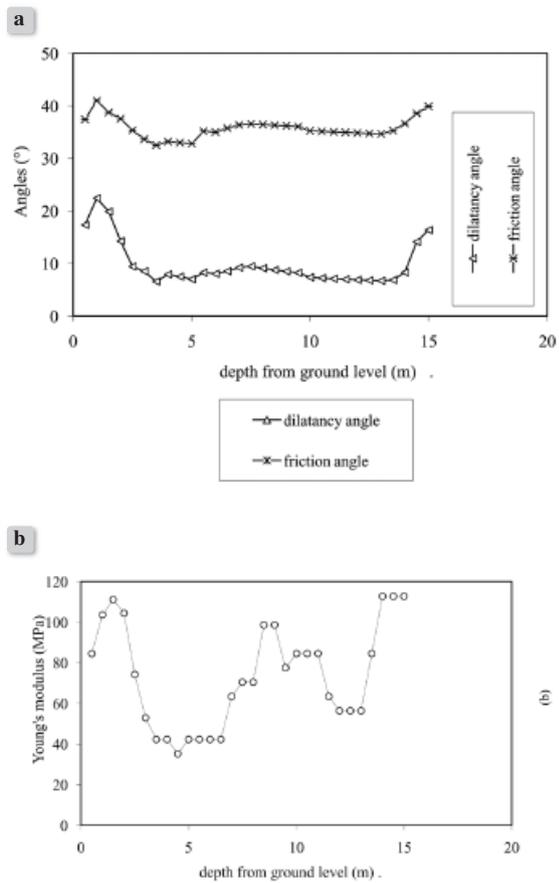
**Figure 7.** Profiles of friction and dilatancy angles (a) and Young's modulus (b)
