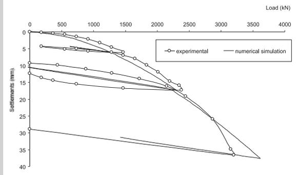
**Figure 8.** Comparison between experimental and calculated load settlement curves (test P3)
