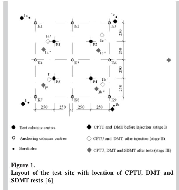
Figure 1. Layout of the test site with location of CPTU, DMT and SDMT tests [6]
