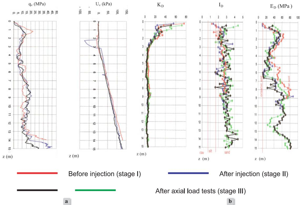
Figure 2. Sample of in situ test results a) CPTU test; b) DMT test [6]
