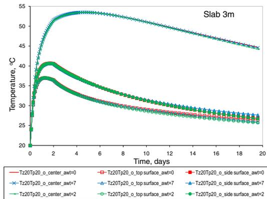
**Figure 3.** Temperature distribution in the slab s\_3m over the curing period for different value of coefficient  $\alpha_{WT}$  ( $\text{awt}$  denotes  $\alpha_{WT} \times 10^{-11}$ )
