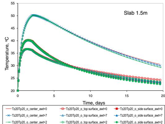
**Figure 4.** Temperature distribution in the slab s\_1.5m over the curing period for different value of coefficient  $\alpha_{WT}$  ( $\text{awt}$  denotes  $\alpha_{WT} \times 10^{-11}$ )
