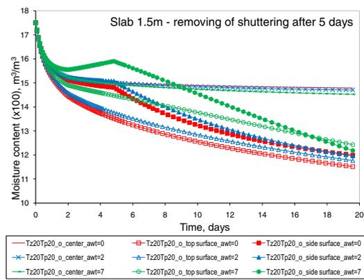
Figure 10. Moisture distribution in the slab s\_1.5m\_r\_5 over the curing period for different value of coefficient  $\alpha_{WT}$  (awt denotes  $\alpha_{WT} \times 10^{-11}$ )
