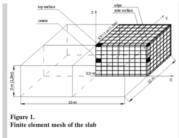
Figure 1. Finite element mesh of the slab
