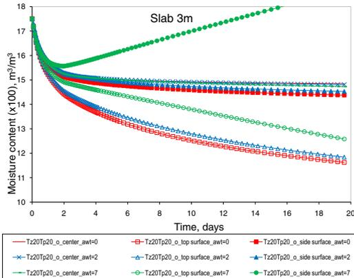
Figure 7. Moisture distribution in the slab s\_3m over the curing period for different value of coefficient  $\alpha_{WT}$  (awt denotes  $\alpha_{WT} \times 10^{-11}$ )
