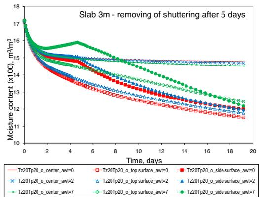
Figure 9. Moisture distribution in the slab s\_3m\_r\_5 over the curing period for different value of coefficient  $\alpha_{WT}$  (awt denotes  $\alpha_{WT} \times 10^{-11}$ )
