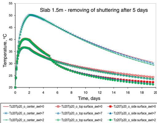
Figure 6. Temperature distribution in the slab s\_1.5m\_r\_5 over the curing period for different value of coefficient  $\alpha_{WT}$  (awt denotes  $\alpha_{WT} \times 10^{-11}$ )
