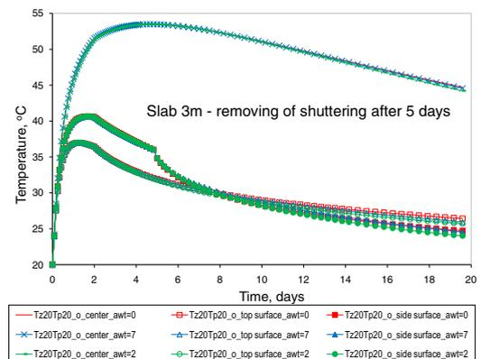
**Figure 5.** Temperature distribution in the slab s\_3m\_r\_5 over the curing period for different value of coefficient  $\alpha_{WT}$  ( $\text{awt}$  denotes  $\alpha_{WT} \times 10^{-11}$ )
