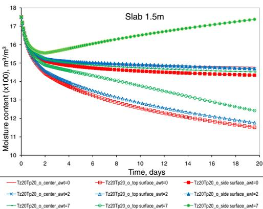
Figure 8. Moisture distribution in the slab s\_1.5m over the curing period for different value of coefficient  $\alpha_{WT}$  (awt denotes  $\alpha_{WT} \times 10^{-11}$ )
