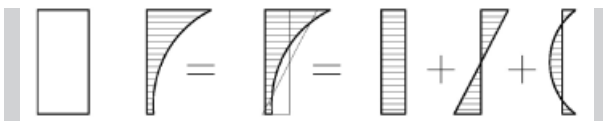
Figure 4. Temperature or thermal strain in cross-section of an element, for unsteady heat flow
