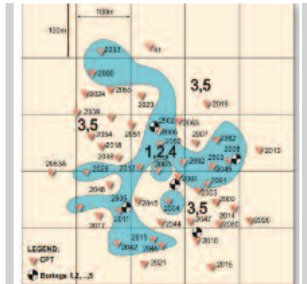
Figure 21. Subsoil division on agglomerations of CPT according to the centroid method
