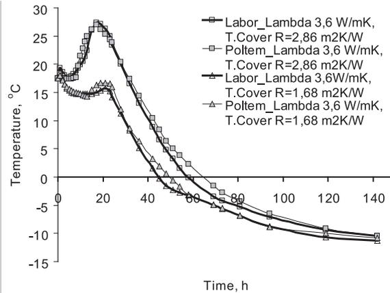
Figure 3. Comparison of surface and computational distribution of temperature for curing concrete in pole elements of small massiveness  $M_p=40^1$ , depending on the employed heat conduction coefficient [POLTEM]
