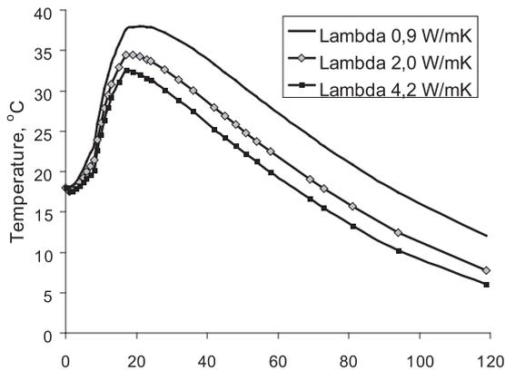
Figure 2. Computational temperature (POLTEM) in curing concrete nucleus depending on employed heat conducting coefficient
