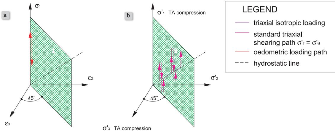
Figure 1. Loading paths feasible in standard tests in: a) a conventional triaxial apparatus, b) an oedometer
