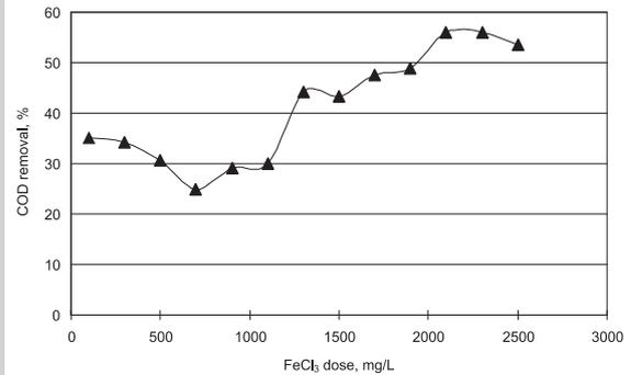
Figure 1. COD removal from landfill leachate using  $\text{FeCl}_3$
