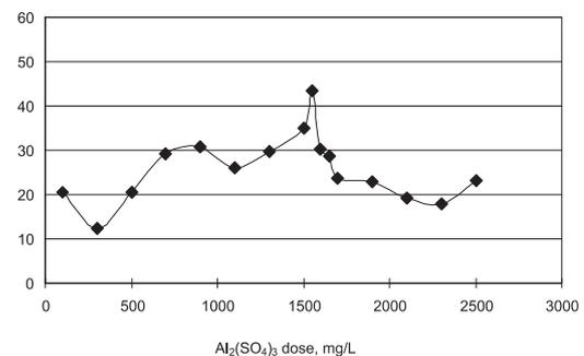
Figure 3. COD removal from landfill leachate using  $\text{Al}_2(\text{SO}_4)_3$
