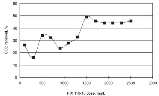
Figure 2. COD removal from landfill leachate using PIX 110-10
