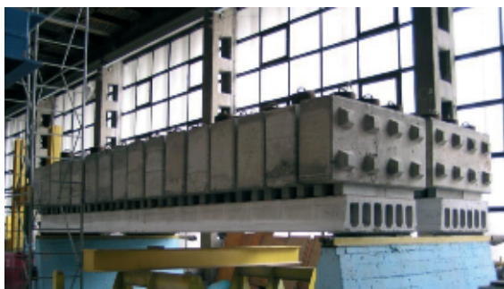
Figure 3. HCS-3 and HCS-4 slabs subjected to long-term loading
