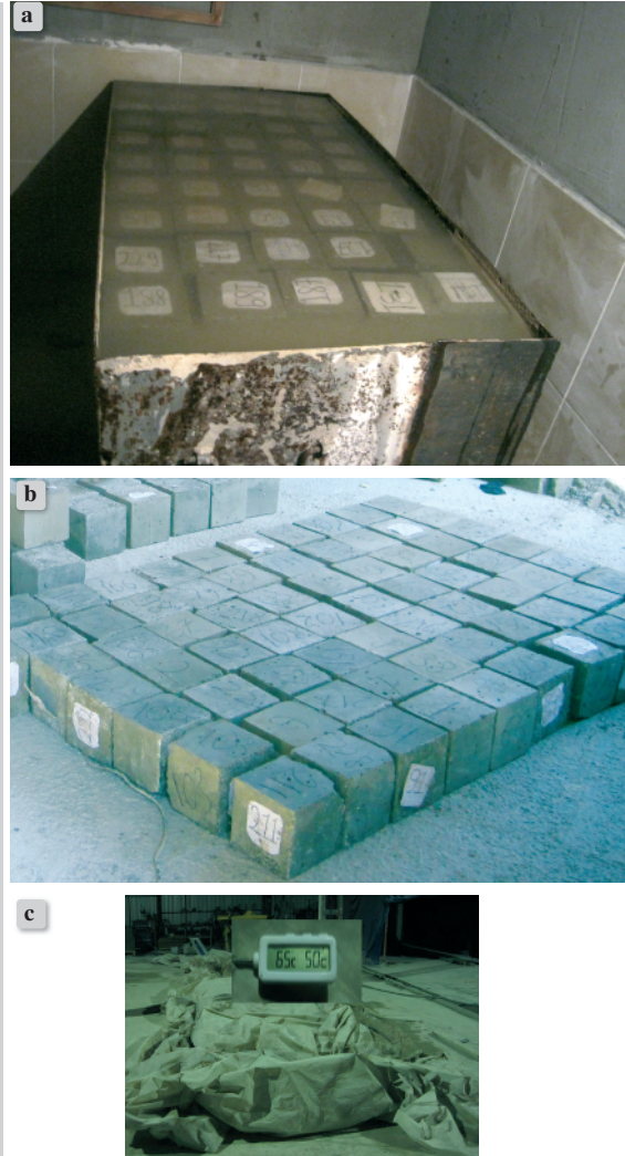
Figure 2. a) water, b) air and c) steam curing
