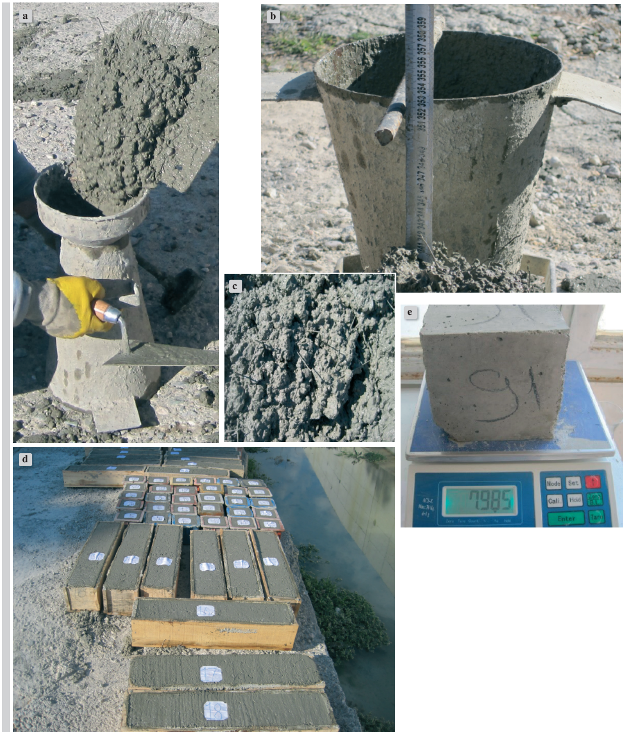
Figure 5. Workability tests (a-c); mixtures in molds (d); weights of specimens (e)
