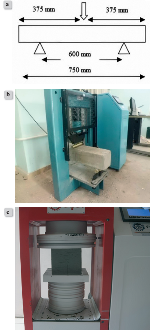
Figure 4. Mechanical testing of specimens a) Schematic demonstration of flexural tests; 375 mm (14.76 inches), 600 mm (23.62 inches) 750 mm (29.52 inches) b) Flexural tests c) Compression tests
