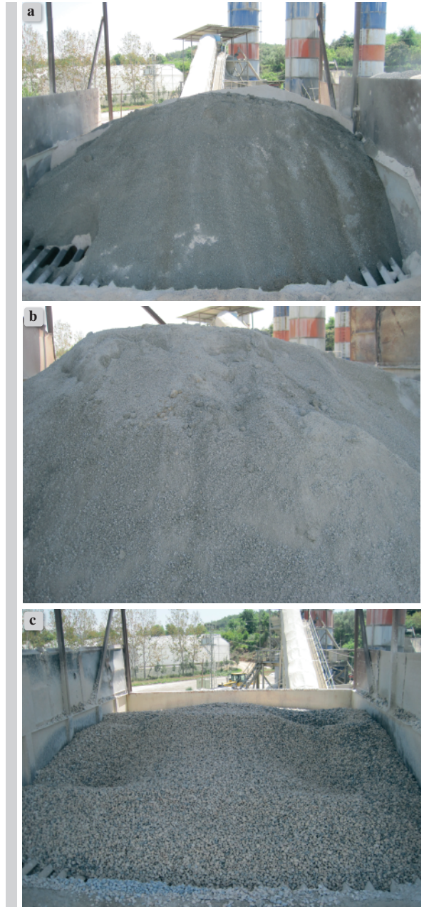
Figure 1. Aggregates for each size; a) 0–4 mm b) 4–12 mm c) 12–22 mm
