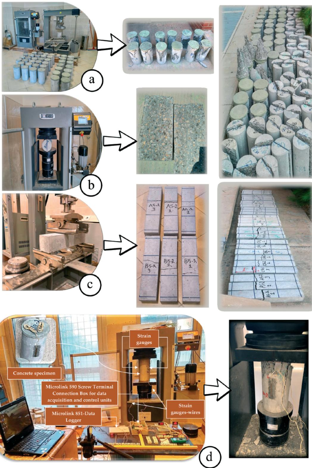
Figure 5. Pictures showing the sides of the tests carried out on hardened concrete modified with and without GP. (a) Samples being prepared and tested for their compressive strength; (b) splitting tensile strength test; (c) flexural tensile strength test; (d) test configuration for modulus of elasticity
