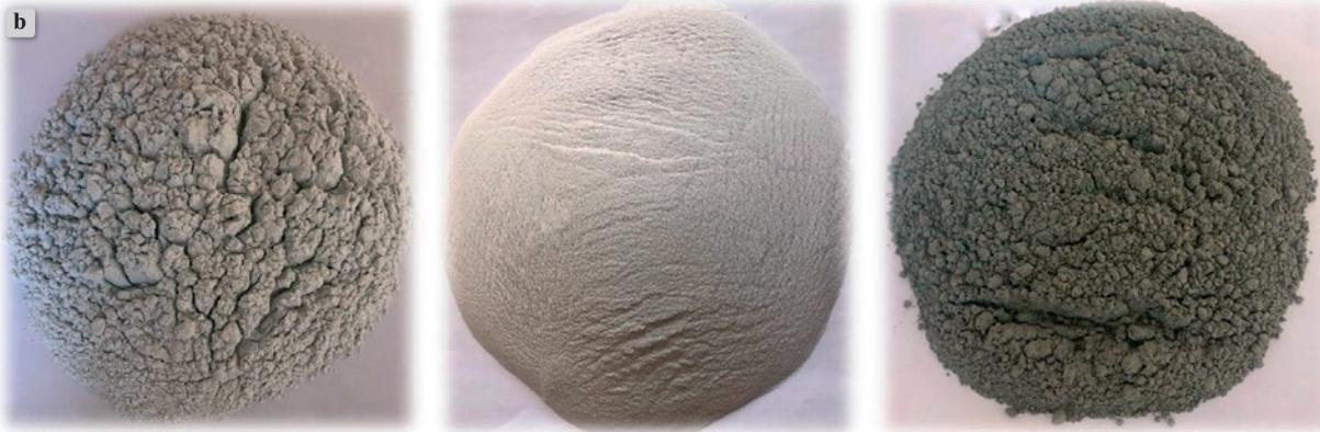
Figure 2. (a) Particle size distribution curves of cement, GP-A, and GP-B, (b) waste glass powder after milling and cement used in the study
