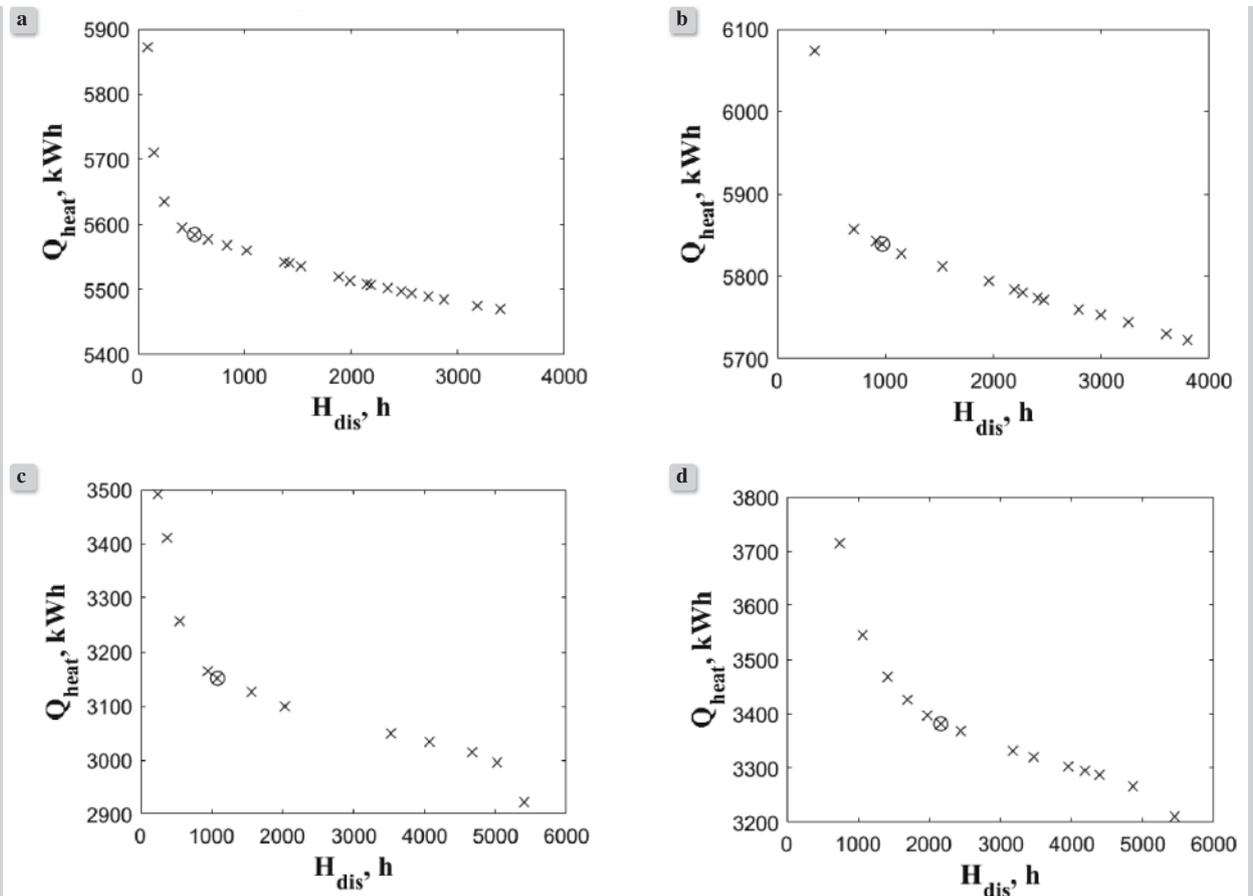
Figure 3. Pareto Front: a) brick standard building, b) wood standard building, c) brick passive building, d) wood passive building
