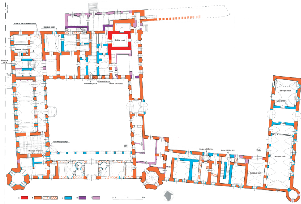
Figure 9a. Żyrowa, the palace, ground floor plan with chronological stratification of walls. Legend: A – Gothic (the 15 th century); B – Mannerism (1631–1644) (walls: found, presumed, foundation benches); C – Baroque (1781); D – approx. 1899; E – 1905–1911; F – walls unknown and from the 20 th century; RC – stately courtyard; GC – garden courtyard (edited by Authors)
