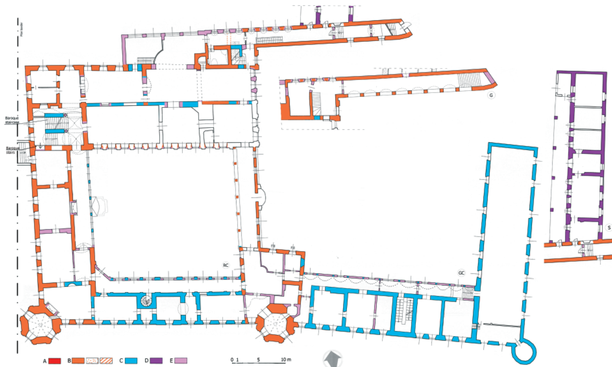
Figure 9b. Żyrowa, the palace, first floor plan with chronological stratification of walls. Legend: A – Gothic (the 15 th century); B – Mannerism (1631–1644); C – Baroque (1781); D – approx. 1899; E – 1905–1911; F – walls unknown and from the 20 th century; RC – stately courtyard; GC – garden courtyard; G – Gallery second level; S – shed; (edited by Authors)
