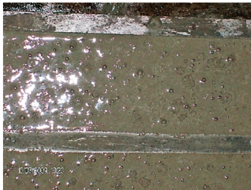
Figure 2. View of the self-compacting process of mortar incorporating PCP and AFA
