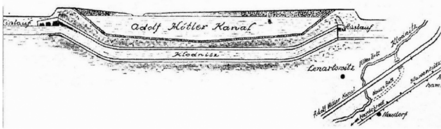
Figure 3. The cross-section of the crossing and the location of the Kłodnica River [16]
