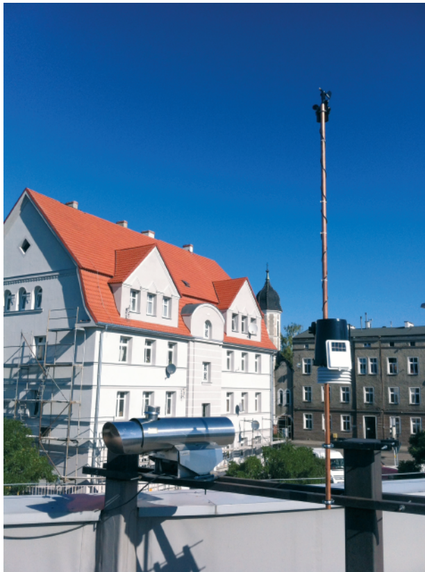
Figure 3. A photo of the light beam transmitting and receiving device
