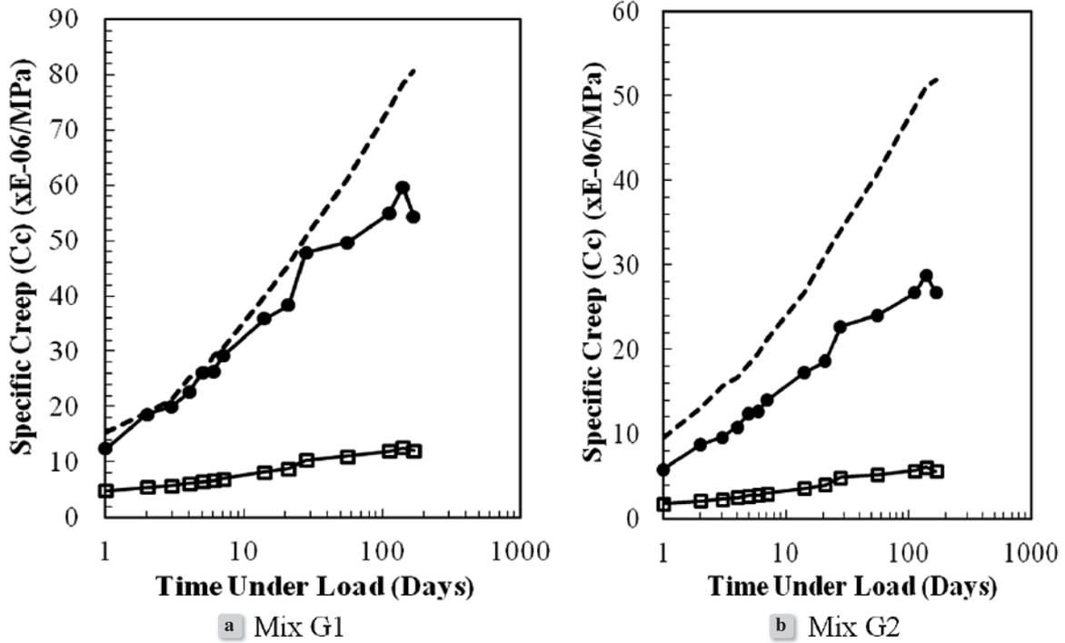
Figure 2. Measured and predicted specific creep for granite concretes
