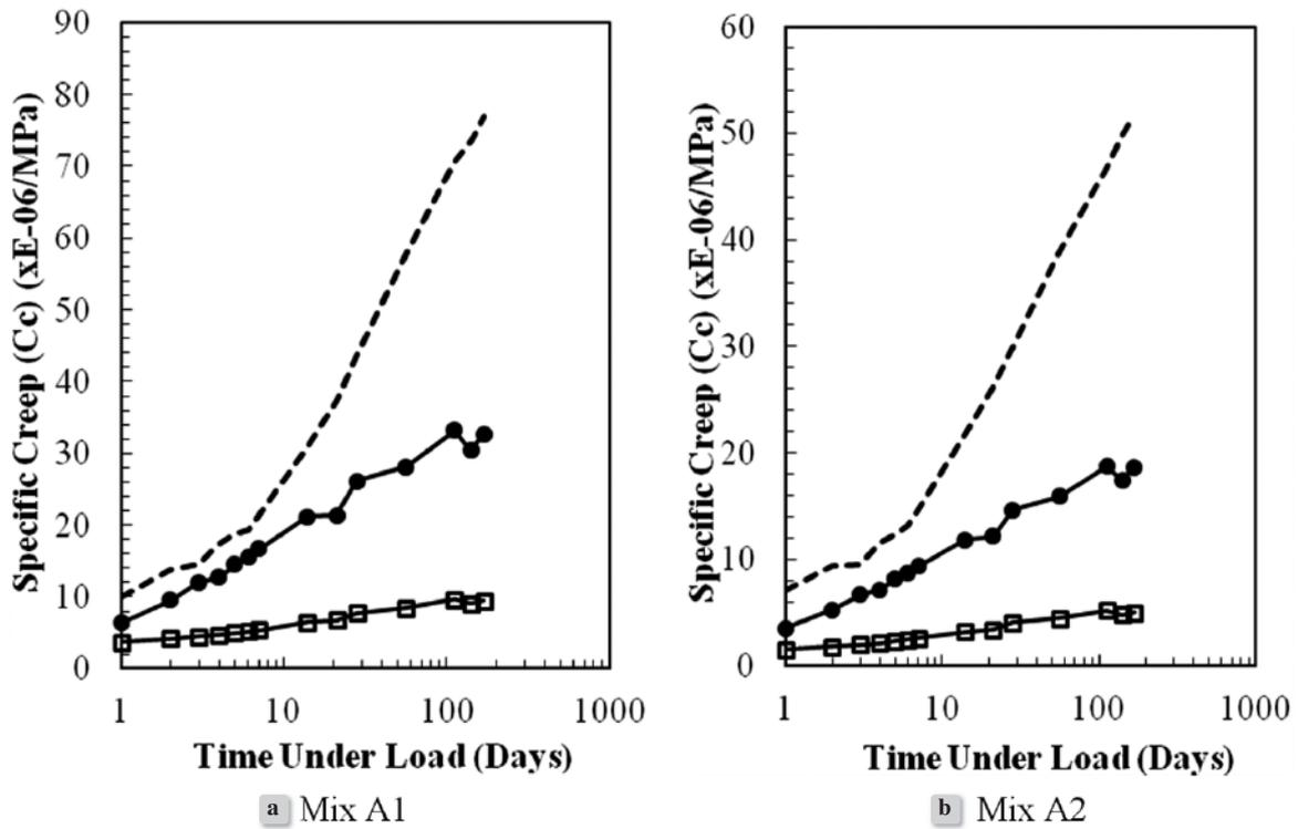
Figure 3. Measured and predicted specific creep for andesite concretes
