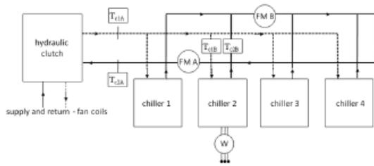
**Figure 2.** The scheme of the cooling system in the building 1 with marked location of the measurement points: cooling capacity of chillers group – flow meter FM A, temperature sensors  $T_{c1A}$ ,  $T_{c2A}$ ; cooling capacity of the chiller 2 – flow meter FM B, temperature sensors  $T_{c1B}$ ,  $T_{c2B}$ ; electric power of the chiller 2 – electric power meter W
