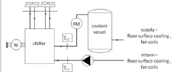
**Figure 4.** The scheme of the cooling system in building 2 with marked location of the measurement points: measurement of cooling capacity of the chiller – flow meter FM, temperature sensors  $T_{c1}$ ,  $T_{c2}$ , measurement of the delivered electric power – electric power meter W
