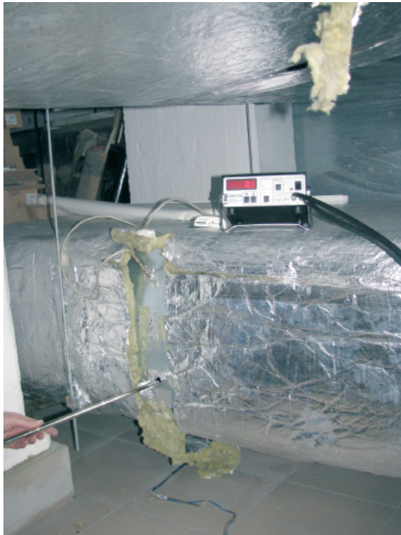
Figure 6. Measurement of pressure distribution in the ventilation duct using a Prandtl tube
