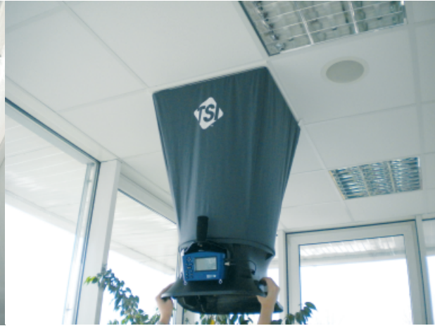
Figure 11. Measurement in the supply channel by means of a Prandtl tube and measurement of ventilation air volume flow using a balometer
