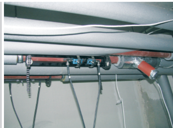
Figure 8. Measurement of the flow volume of heating water by the use of an ultrasonic flow meter and the flow temperature of the heater by the use of an adhesive thermometer
