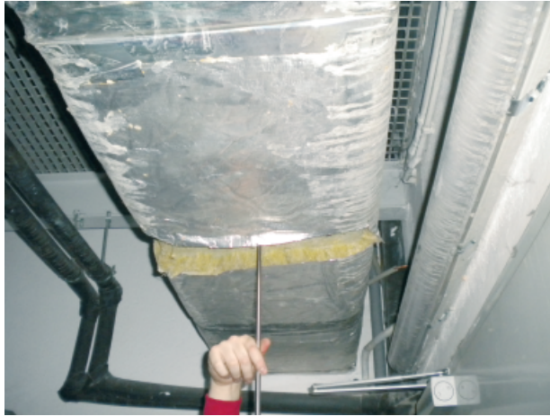
Figure 11. Measurement in the supply channel by means of a Prandtl tube and measurement of ventilation air volume flow using a balometer
