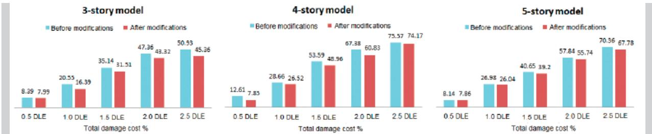
**Figure 6.** Percentage of total damage cost for models with different number of stories before and after conducting the proposed modifications for components' distribution in height
