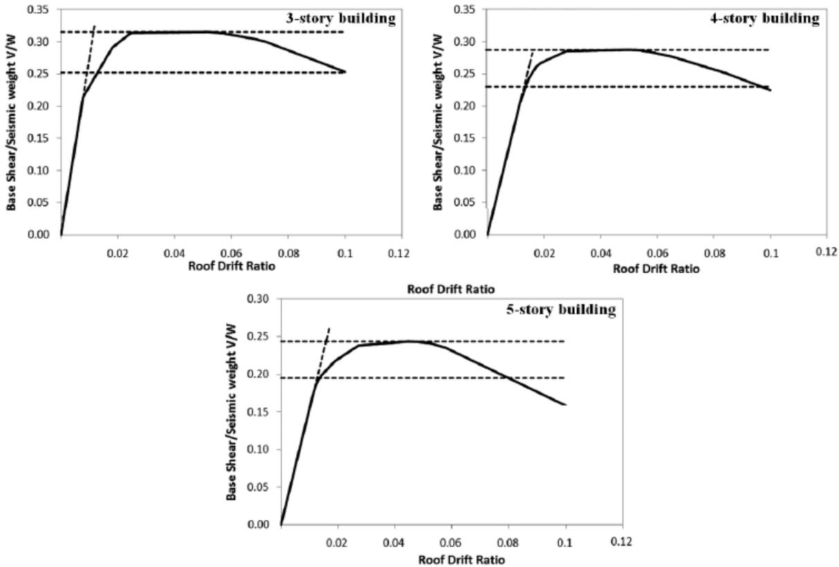
Figure 5. Pushover diagrams for different models
