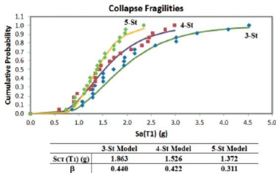
Figure 3. Collapse fragilities of the models
