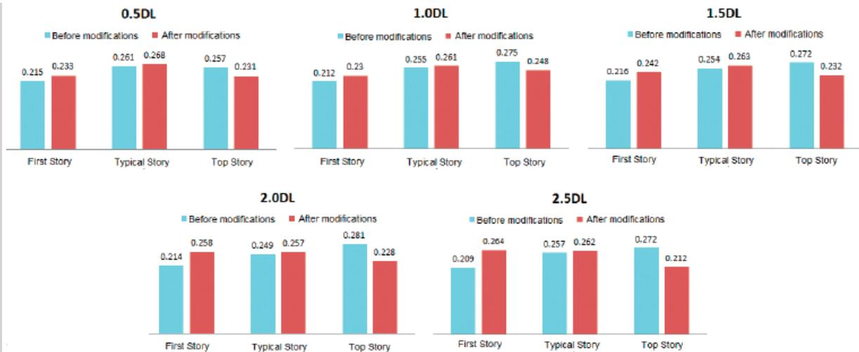
Figure 8. Percentage of incorporation of stories in total damage cost for 4-story model subjected to different scaling intensity levels for two alternative nonstructural distributions
