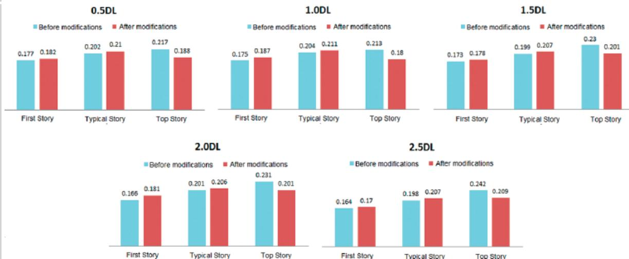
Figure 9. Percentage of incorporation of stories in total damage cost for 5-story model subjected to different scaling intensity levels for two alternative nonstructural distributions
