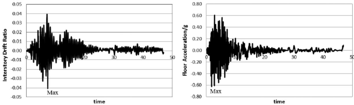
Figure 4. Structural responses of the roof story in 3-story model in scaling level of 1.5 DLE
