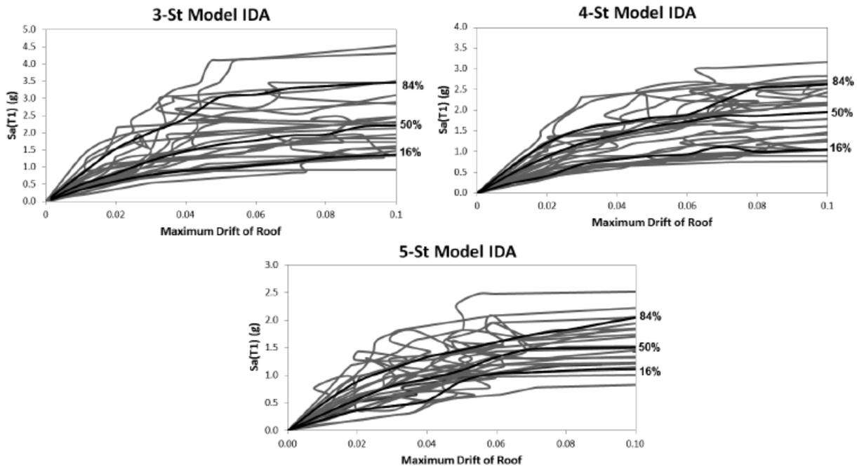
Figure 2. Incremental dynamic analysis results, spectral acceleration amount according to maximum drift of the roof story, for different models
