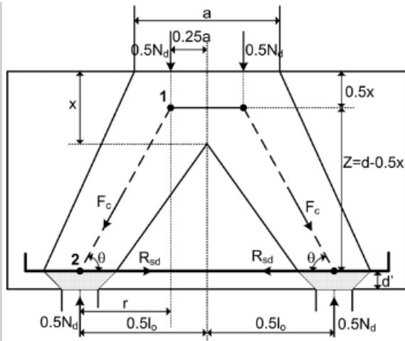
Figure 4. Proposed strut-and-tie model for two-pile caps
