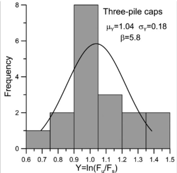
Figure 11. Histogram for three-pile caps
