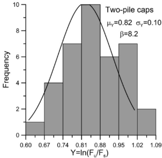
Figure 9. Histogram for two-pile caps
