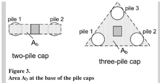
Figure 3. Area  $A_b$  at the base of the pile caps
