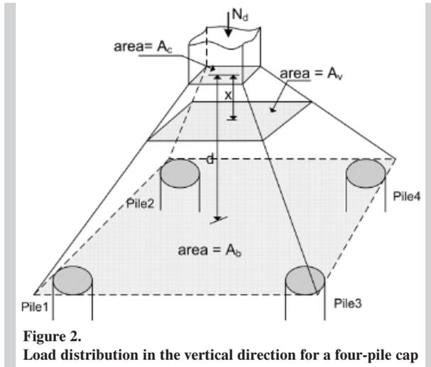
Figure 2. Load distribution in the vertical direction for a four-pile cap
