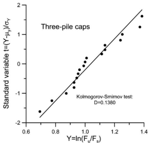
Figure 10. Probability paper for three-pile caps
