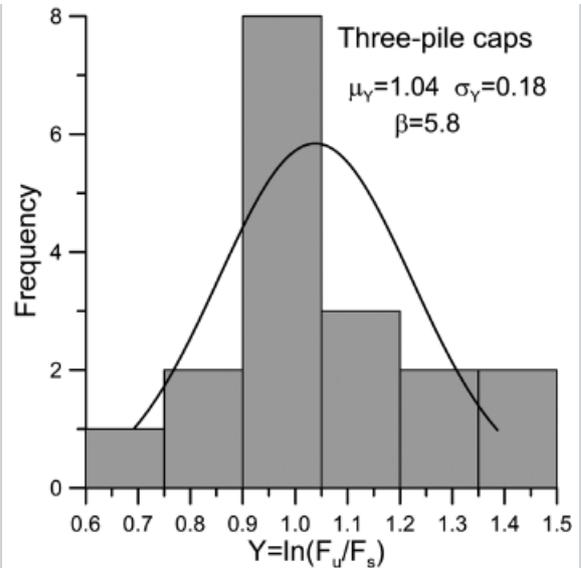
Figure 11. Histogram for three-pile caps
