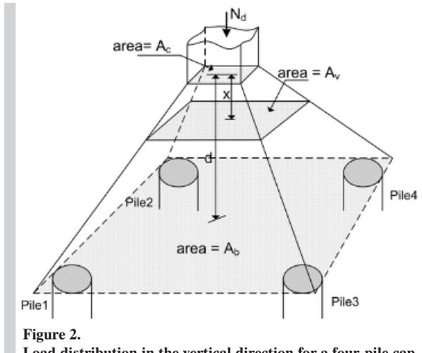
Figure 2. Load distribution in the vertical direction for a four-pile cap
