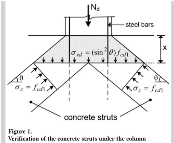
Figure 1. Verification of the concrete struts under the column
