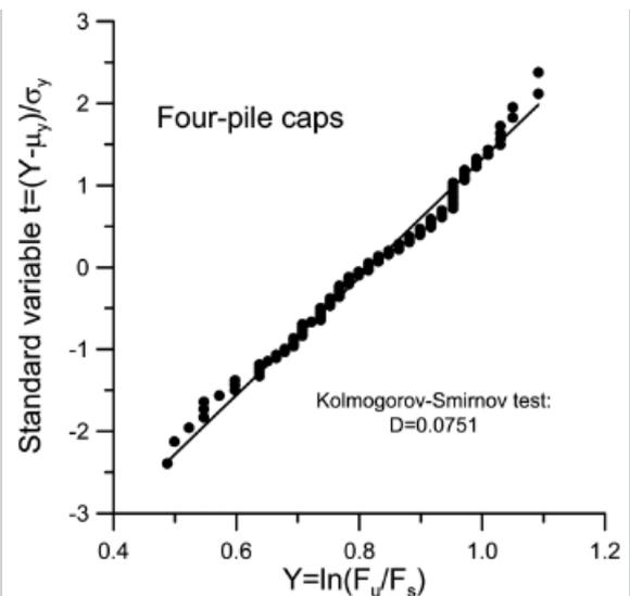
Figure 12. Probability paper for four-pile caps
