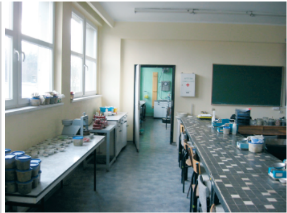
Figure 6. Room 119L (Classroom) for examination of soil physical parameters: on the right side working tables with Cassagrande apparatuses; further, way to room; (photo by Joanna Tymkiewicz)
