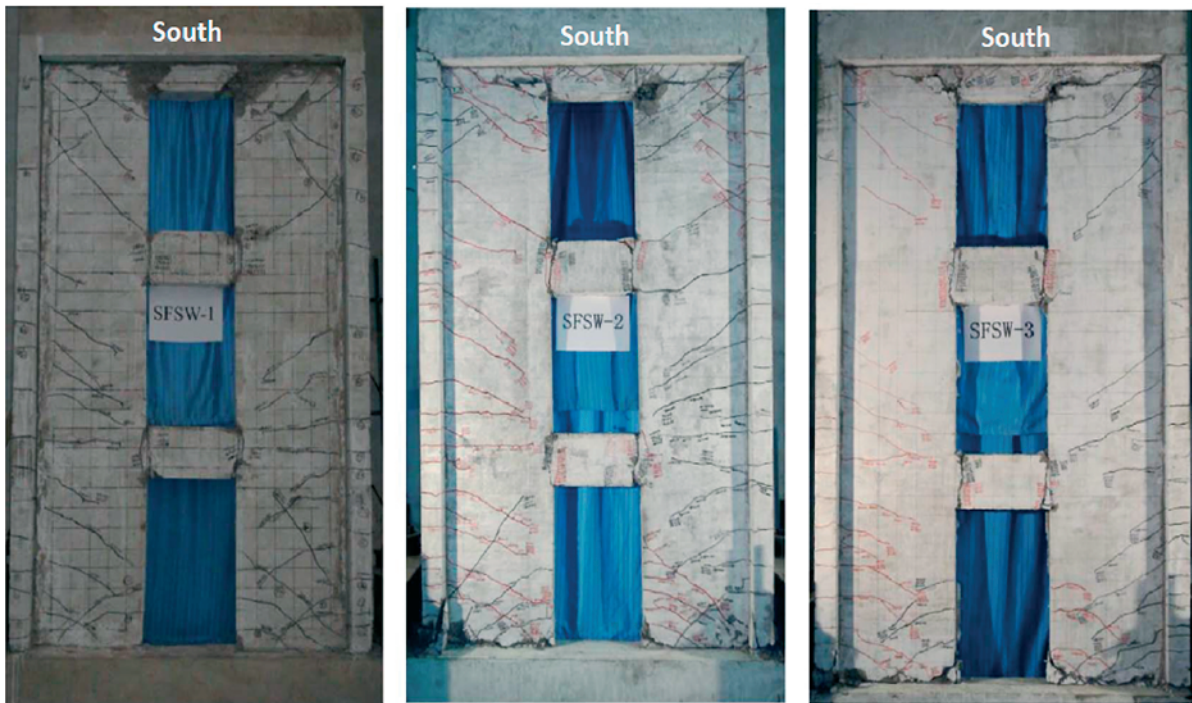
Figure 11. Crack patterns of CSWs [56]
