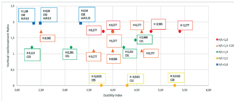
H: Horizontal reinforcement ratio, C: Concrete compressive strength, ALR: Axial load ratio ( ALR=N/f_c b_w t )
